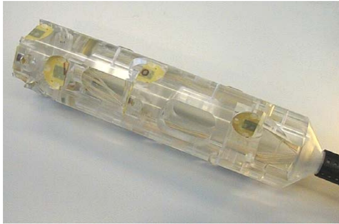
Figure 4. Photograph of one of 19 identical modules of the 304 SQUID vector magnetometer system.
